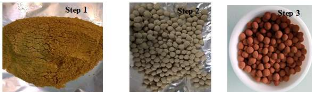
Figure 1. Steps in the manufacture of calcined clay beads. Source: Authors
